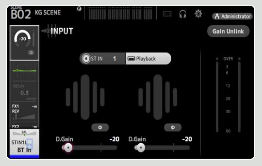
To enable USB playback, change the INPUT of the Stereo In to "Playback" via the channel's GAIN settings
