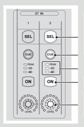
Each console has two Stereo Inputs fed by RCA jacks
